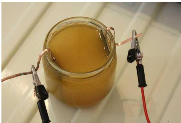
*After etching has stopped the precipitate starts to fall to the bottom as it is formed by the reaction between cupric chloride and caustic soda*
