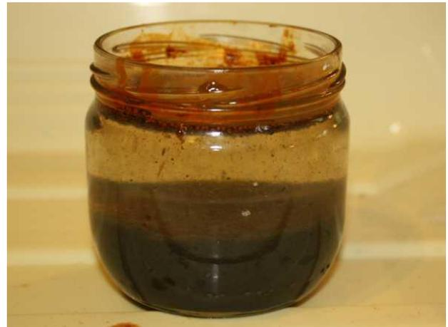
*Etching Aluminium anode in brine – the aluminium is slow to react with the chlorine which can be seen as bubbles being given off the anode plate and a thick foam forms very rapidly on the surface trapping bubbles of hydrogen and chlorine.*
