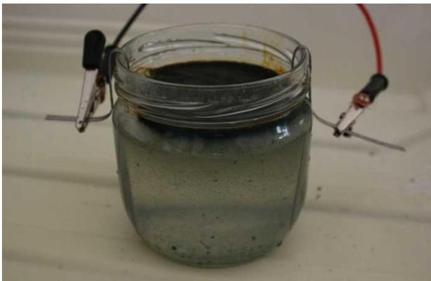
*Etching steel (iron anode) in brine – black foam forms on the surface very rapidly. The bubbles are formed by hydrogen in caustic soda and ferric chloride.*
