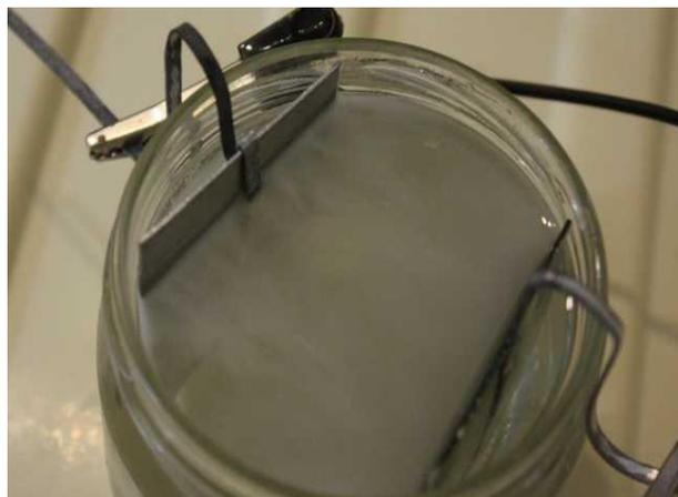
*Stainless steel should not be used as an anode, because it is very resistant to being etched, or in other words, it will not combine easily with the Chlorine, which is either given off as a gas, or reacts with the caustic soda to produce Sodium Chlorate, which is a weed killer now banned for use in the European Union.*
