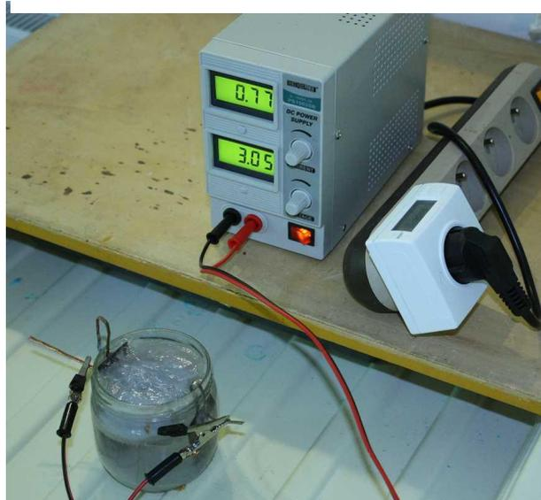
instance platinum or carbon) it will not react with the Chlorine ions, and the gas will be given off as bubbles and can be separated and collected. The positive Sodium ions will react with water rather than with the negative metal of the cathode (explained below) releasing hydrogen as gas. The water ( $H_2O$ ) loses an ion of hydrogen leaving  $HO$  which combines with the Sodium to make Sodium Hydroxide (Caustic Soda).
