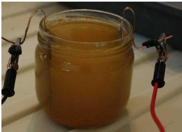
reactions are produced by Zinc, Iron, or Aluminium used as anodes, producing Zinc(II)Chloride, Iron(III)Chloride, or Aluminium(III)Chloride, and then reacting with the caustic soda, to leave Zinc Hydroxide (grey), Iron Hydroxide (black), or Aluminium Hydroxide (white).
